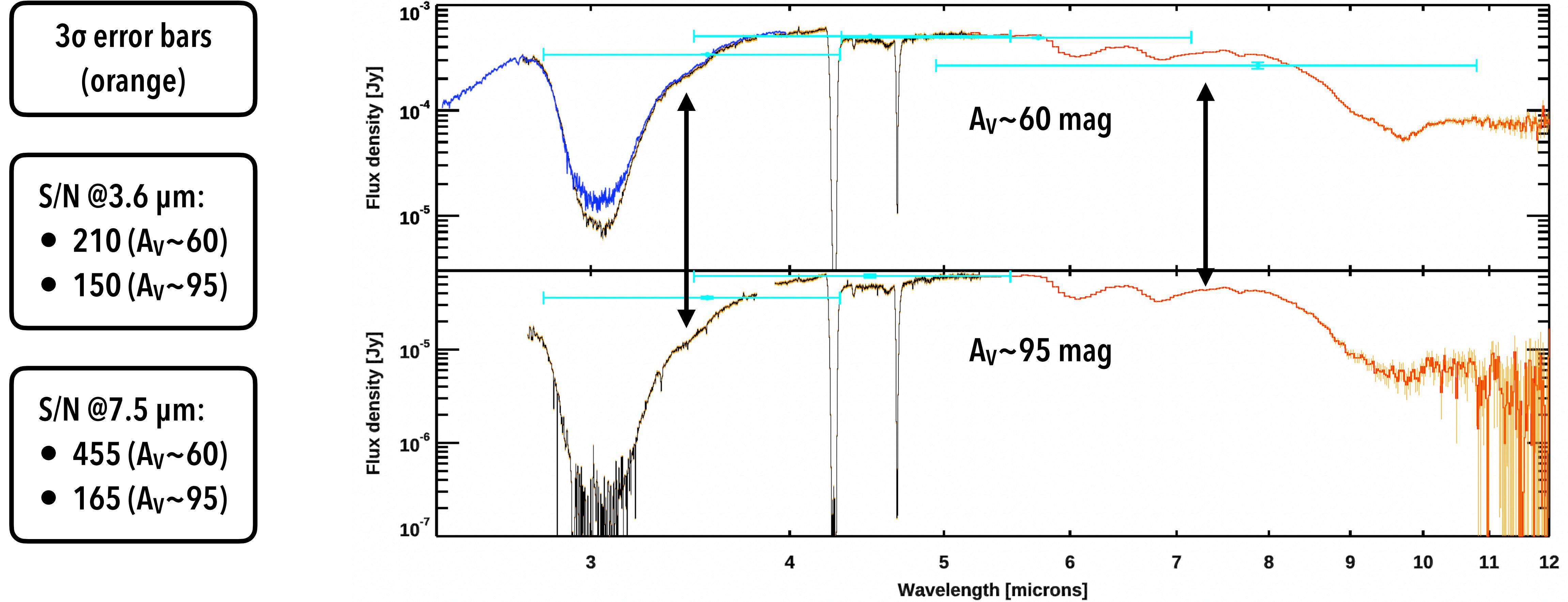
Able to detect 0.2  $\mu$ Jy in wings of  $A_V \sim 95$  spectrum H<sub>2</sub>O feature
